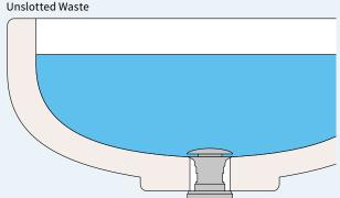
If your basin has a built-in overflow, you will need a SLOTTED basin waste which will allow overflow water to be drained, whether the waste is open or not.
